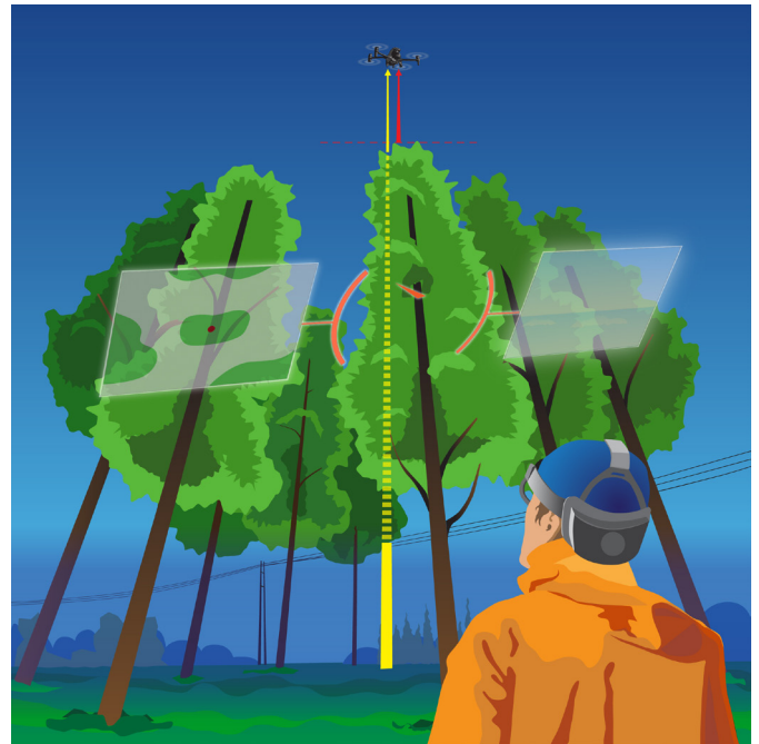
Fig. 4 - Height indicators, including ultrasound / camera-based short range detection, are always shown, even when flying partially or totally beyond visual line of sight
